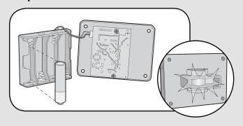
Install 4 AA Alkaline batteries (not provided). (Lithium batteries recommended for colder environments.) Test light will flash.
